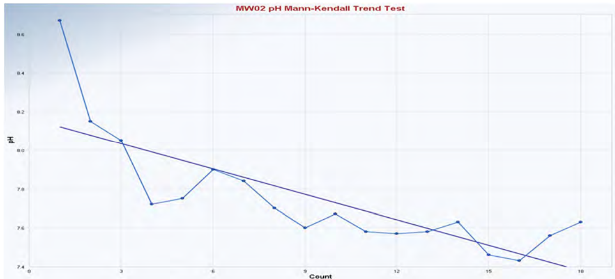
Figure 5 Statistical trend analysis for pH levels at MW02
