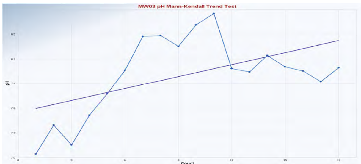
Figure 6 Statistical trend analysis for pH levels at MW03
